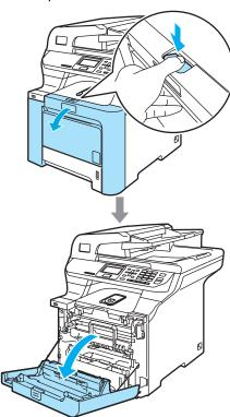
Hold the green handle of the drum unit. Lift the drum unit up and then pull it out until it stops.
